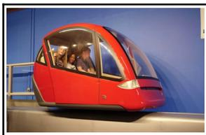
**Slide 8** shows an AVT vehicle with a carrying capacity that puts it in the medium-sized GRT category. PRT vehicles are much smaller and - most importantly - much lighter weight. The ITNS (Intelligent Transportation Network System) version of PRT (shown on the left)
