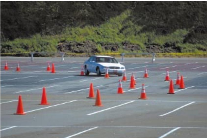
*Fully automated LeSabre corners on PATH test track.*
